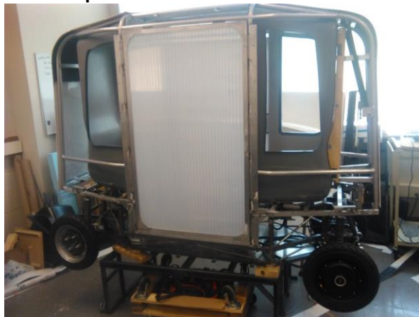
One of the changes from Version 1 to Version 2 is the addition of in-wheel motors. These pictures show the testing of the motor (located in the hub of the wheel).
