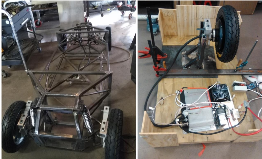
Welded Frame of Version 2 Vehicle. In-wheel motors are located in the rear wheels in the hub.
