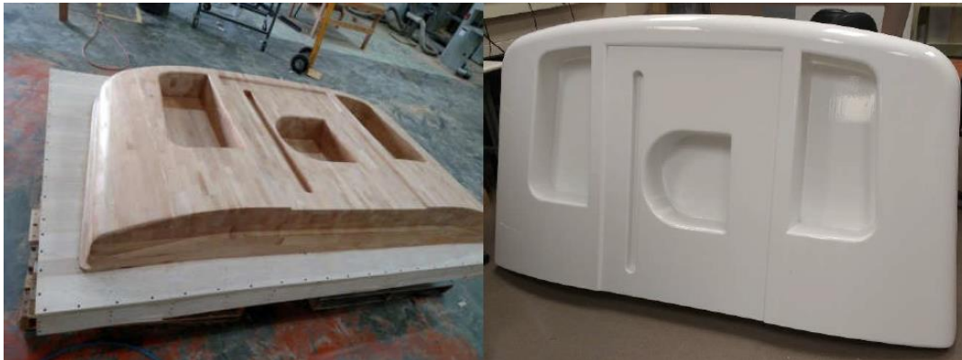
Mold (on left) was used to thermo-form shell part (on right).
